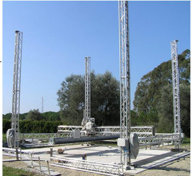
The Contour Crafting system is a robot that automates tools normally used by hand. These are wielded by a robotic gantry that builds a three-dimensional object.
